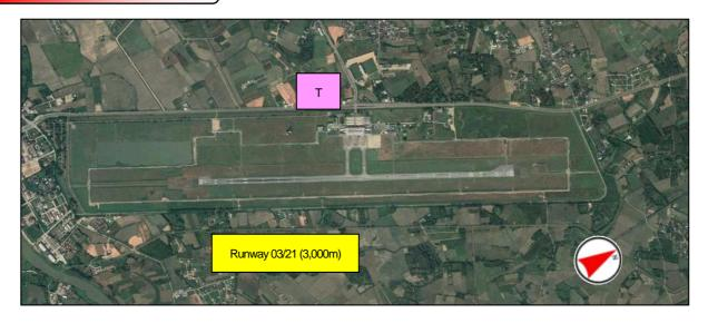
The airport is at an elevation of 390m above mean sea level. It has one runway designated 03/21 with an asphalt surface measuring 3,000m by 45m.
