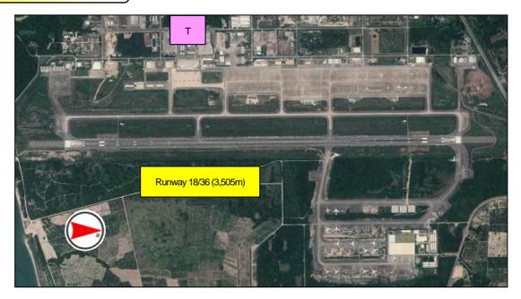
The airport is at an elevation of 13m above mean sea level. It has one runway designated 18/36 with an asphalt surface measuring 3,505m by 45m.
