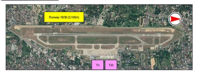
The airport is at an elevation of 316m above mean sea level. It has one runway designated 18/36 with an asphalt surface measuring 3,100m by 45m.
